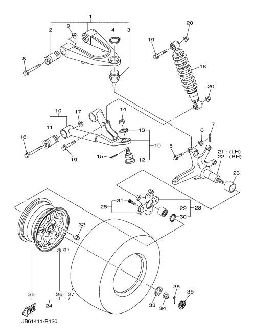
FIG. 3 FRONT SUSPENSION & WHEEL
