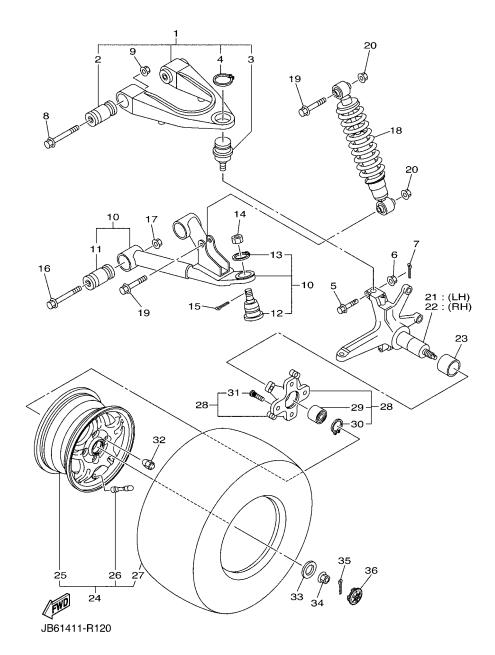
FIG. 3 FRONT SUSPENSION & WHEEL
