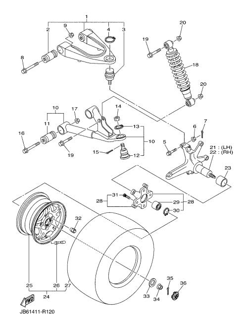
FIG. 3 FRONT SUSPENSION & WHEEL
