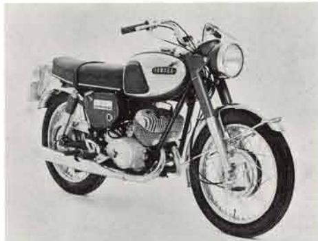
YM 2 C is fitted with unique piston fork damper to minimize shocking on the roughest surface of road.
