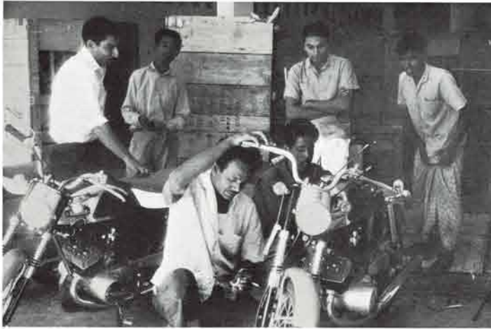
Assembling a Yamaha that has been just delivered.
