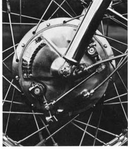
A cap-fitted front double leading-shoe brake is so powerful.
