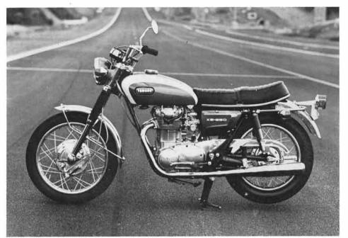
A maximum output of 53 h.p., acceleration of SS 13 sec. for 1/4 mile, top speed of over 185 km/h, these are figures specified in its technical data for the domestic market. They are far above the standard levels.
