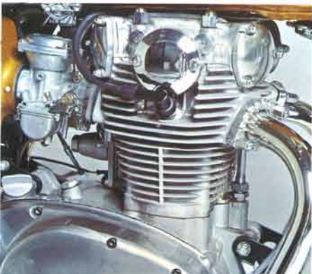
Designed for unmatched performance and superb economy, its powerplant features special wet-sump trochoid pump and twin 33mm constant velocity carburetor for accurate oil supply.
