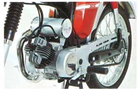
Dependable and powerful 2-stroke rotary valve engine delivers a maximum output of 6hp/9000rpm.
