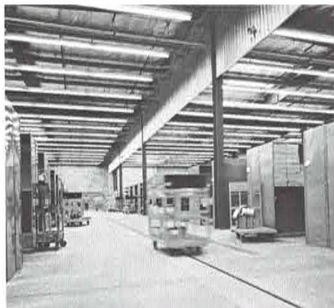
The tow-veyor speeds parts to the shipping area.
