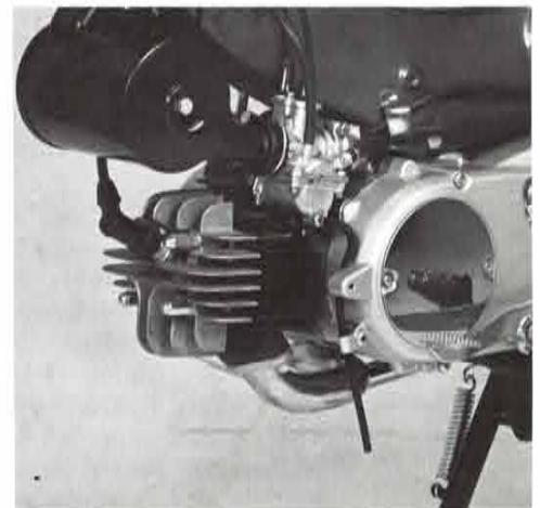
A newly developed reed valve engine assures higher performance.
