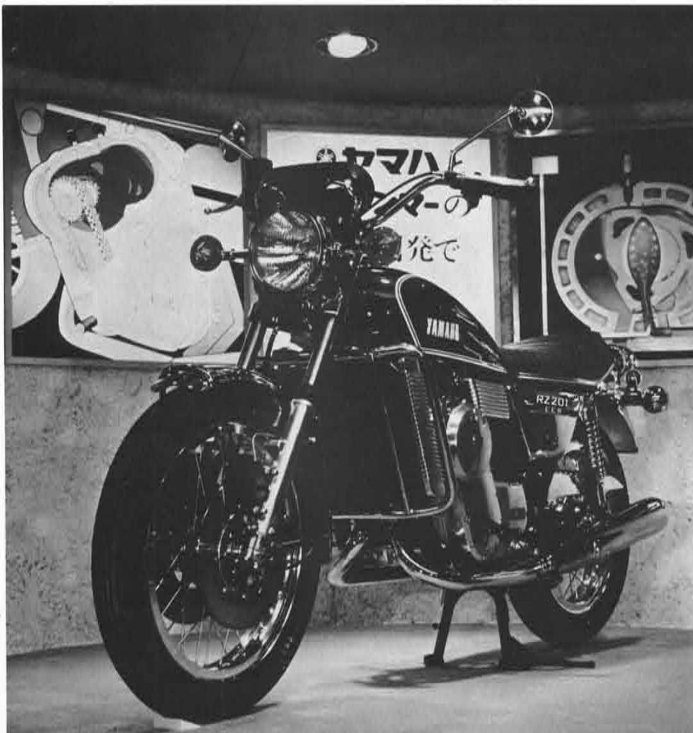
Photo: The Yamaha Rotary RZ201, the first rotary engine motorcycle prototype ever built in the world with the definite intention of mass production, made a quiet but sensational debut at the '72 Tokyo Motor Show. Yamaha has successfully consolidated all proven technical merits into this model, as represented by the in-line twin rotor revolving in the same direction as that of vehicle advance, CCR system, peripheral port, etc. The age of rotarization is about to open with Yamaha.
