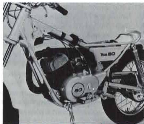
The double-cradle tubular frame has been designed more slim, but, with higher flexible strength, making it ideal for twists and turns in a tough trials section.
