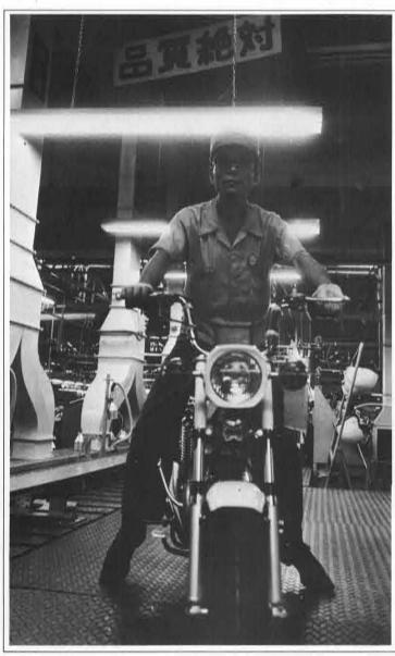
Completion test is one of the most important work processes. Every assembled motorcycle must be thoroughly checked here just before shipment. Four major testing items are sub-divided into 50 points, that's to say, major ones are outlooking, electric equipment, function and cruising. Also, some motorcycles are inspected for power output, fuel consumption, gencharging, erating. lighting, etc. sampling method.
