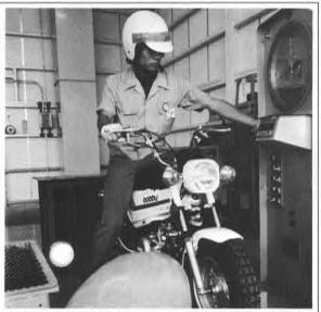
A 50cc Bobby is now placed on a chassis dynamo. Here tested are max. power output, performance curve at low-to-medium speed, fuel and oil consumption.
