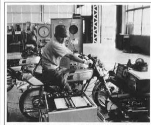
Generating electricity, charging electricity and power consumption are checked against prescribed data. In addition to conducting meter tests, he must always exercise his five senses so that anything imperfect can be detected.
