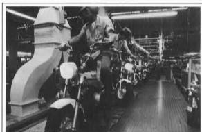
More than 700 component parts are assembled into a Bobby. New bikes are carried onto the line one by one. They are quickly and accurately inspecting those bikes for any loosened bolt, defection bel, starting, gear change, clutch operation, cushioning, etc.
