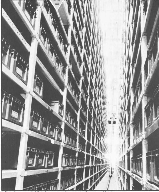
Lofty racks around which 8 stacker cranes are in constant action, are used for storing parts with high turnover rates.
