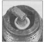
Proper burning: electrode is dry
