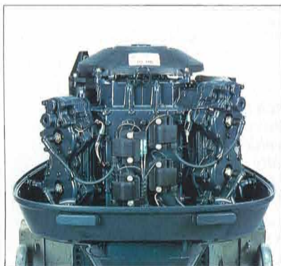
① The new 2-stroke V-4 engine
