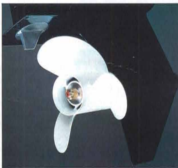
③ The high-speed type lower case and propeller
