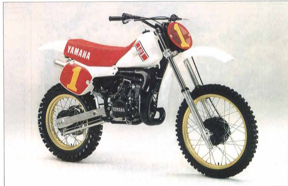
YZM250 •Engine: 2-stroke, water-cooled single •Displacement: 246cc •Max power output: Over 43PS/8,000rpm •Ignition system: C.D.I. •Lubrication system: Pre-mixing (20 : 1) •Transmission: 5-speed gearbox •Tire size (F): 3.00-21 (R): 4.00-18 •Brake (F): Drum (R): Drum •Suspension (F): Telescopic fork (air damper plus coil spring) (R): Swing arm (with Mono-cross unit) •Fuel tank capacity: 9.0 lit •Clutch: Wet multiplate
