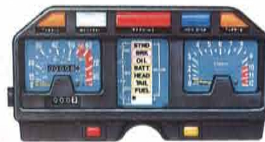
COMPUTERIZED MONITOR SYSTEM
