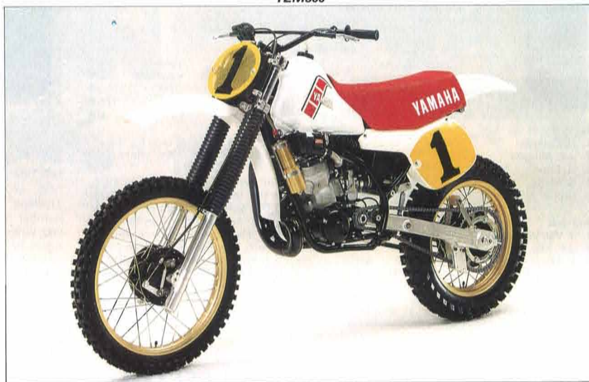
YZM500 •Engine: 2-stroke, water-cooled single •Displacement: 487cc •Max power output: Over 53PS/7,000rpm •Ignition system: C.D.I. •Lubrication system: Pre-mixing (20 : 1) •Transmission: 4-speed gearbox •Tire size (F): 3.00-21 (R): 5.00-18 •Brake (F): Drum (R): Drum •Suspension (F): Telescopic fork (air damper plus coil spring) (R): Swing arm (with Mono-cross unit) •Fuel tank capacity: 11.0 lit •Clutch: Wet multiplate
