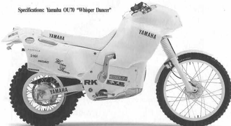
•Engine: Liquid-cooled 2-stroke 200cc •Wheelbase: 1,367mm •Seat height: 830mm •Minimum ground clearance: 268mm •Tire size (front/rear): 2.75-21 — 180/80-14 •Suspension stroke (front/rear): 190mm/175mm •Weight: 120kg
