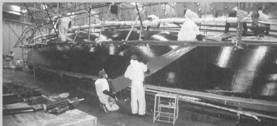
The pre-preg carbon fiber construction method
