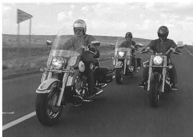
Both the Royal Star (right) and Tour Classic boast a 79 cubic inch V4 powerplant, with smooth shaft drive and classic cruiser styling
