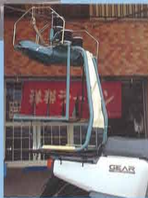
The special okamochi carrier mounted on the back of the bike hangs the load free-swinging from a spring-loaded mounting that smoothes out even bumpy roads to keep the soup from spilling and the pottery bowls from breaking
