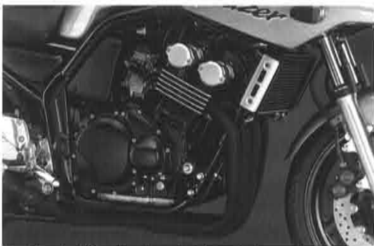
The Fazer's 599cc liquid-cooled four-stroke engine achieves the highest horsepower in the middleweight class
