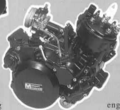
Multi-speed engines like this 50 cc AM 6 are selling mainly to OEM customers
