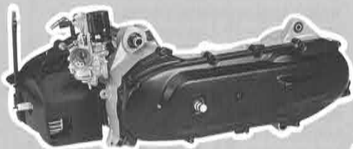
Minarelli's best seller, the 50 cc scooter engine comes in several versions. This is the MY 50 cc horizontal air-cooled engine
