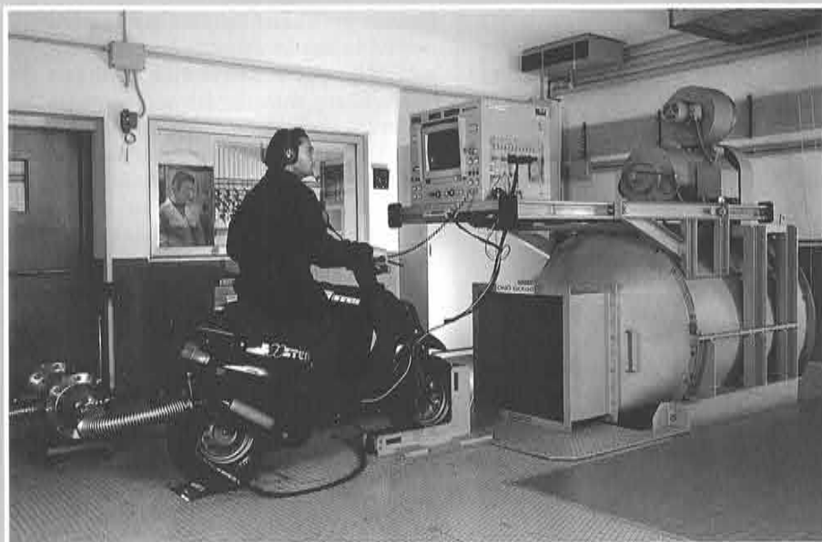
The R&D department's chassis dynamo (test bench)
