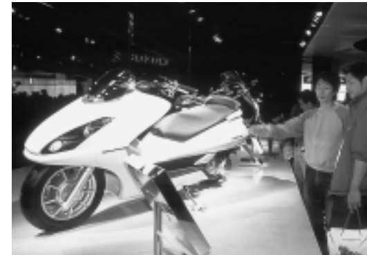
The "MABRICE" features a young "Long & Low" design that is great for tandem riding and sports a unique hybrid drive system. The main rear-wheel drive is provided by the gasoline engine while an electric motor mounted in the front wheel hub gives auxiliary power during acceleration for an even more exciting ride. (Special exhibition model)
