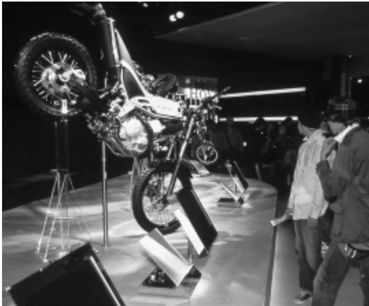
The XG250 Tricker mounts an air-cooled 250cc SOHC single-cylinder engine on a YZ85 size chassis. It gives the image of extreme sports using skateboards or BMX bikes. The special exhibition model "Tricker Pro" displayed along with it is designed to show the possibilities of a true action-riding machine. (Planned Japanese market production model)
