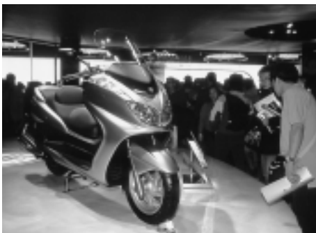
The YP250 Grand Majesty mounts a new-design DOHC 4-valve fuel injection engine on a new frame with 14-inch front and 13-inch rear tires. The engine adopts Yamaha's high-performance DiASil cylinder while the frame makes use of new CF aluminum die-cast parts. (Planned Japanese market production model)
