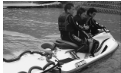
When used as rescue craft, the WaveRunners usually tow a rescue sled
