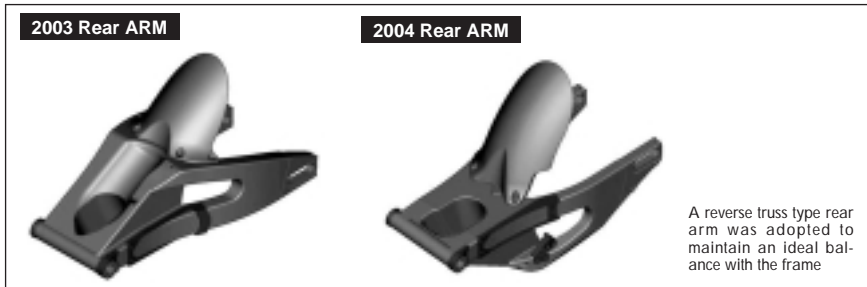
To achieve an optimum rigidity balance with plenty of longitudinal rigidity and more lateral "give," the 2004 model added engine mount arms
